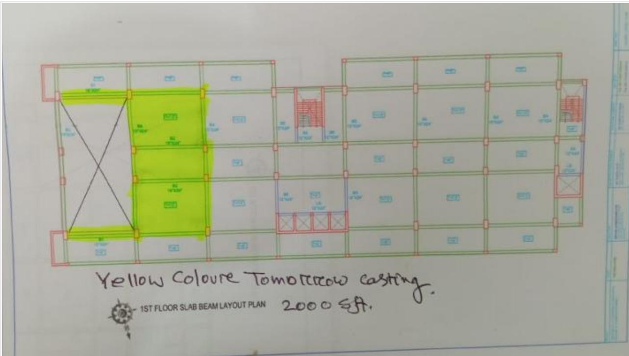
Tower-1-GF Roof Slab-2000 sft Concreting on 21-12-20
