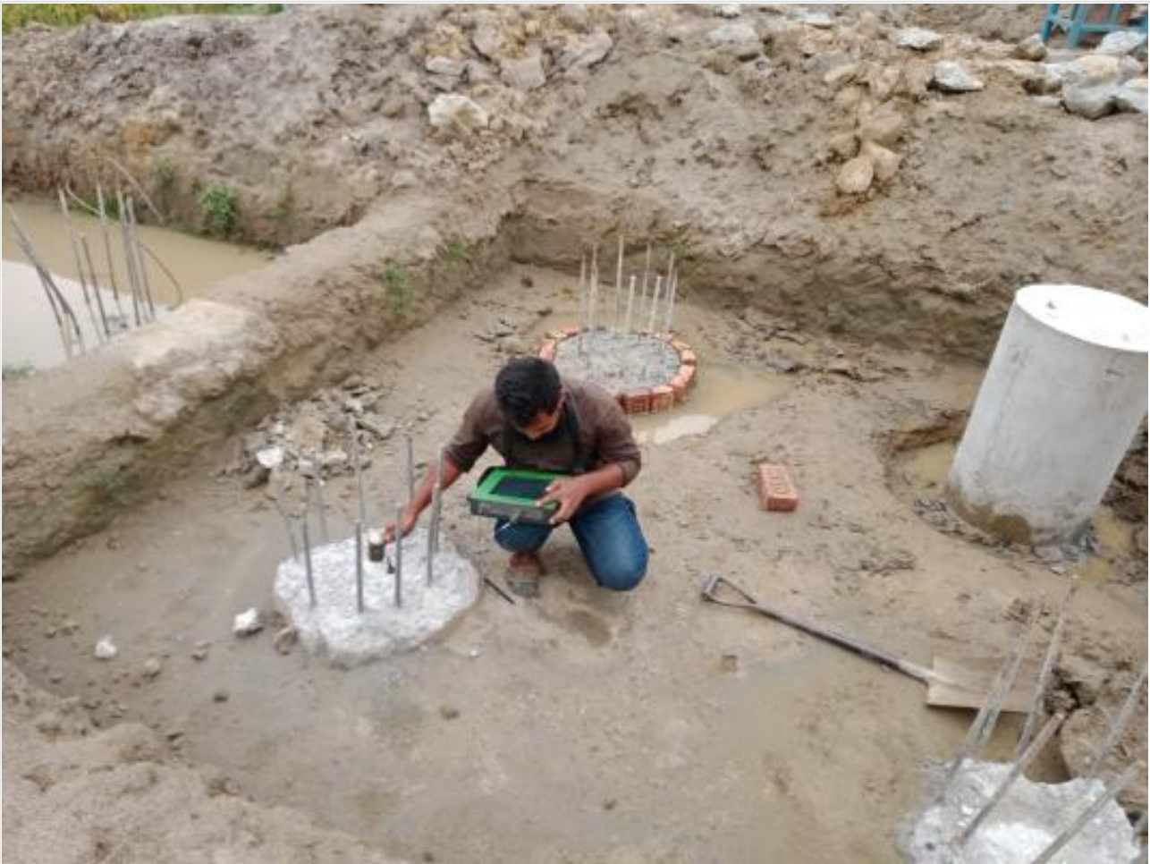
Pile integrity test on 19-05-23
