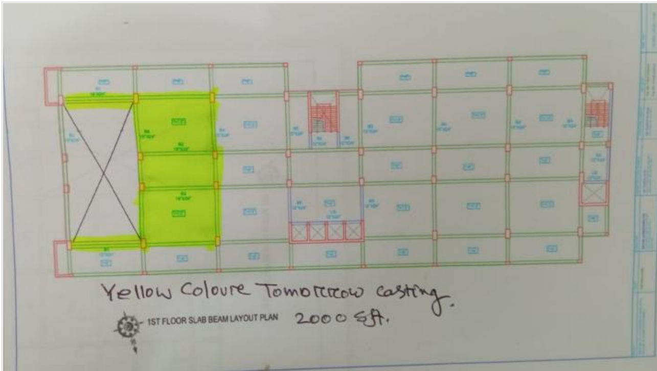
Tower-1-GF Roof Slab-2000 sft Concreting on 21-12-20
